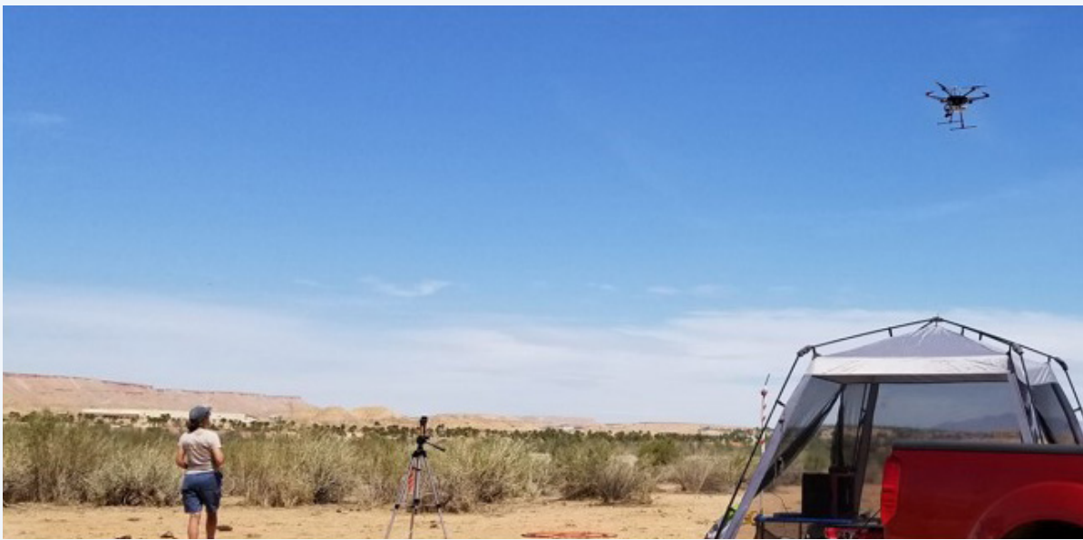
LiDAR Flight. Susan Firor piloting Alta's drone to collect UAS LiDAR data at the Bunkerville riparian reserve unit.
